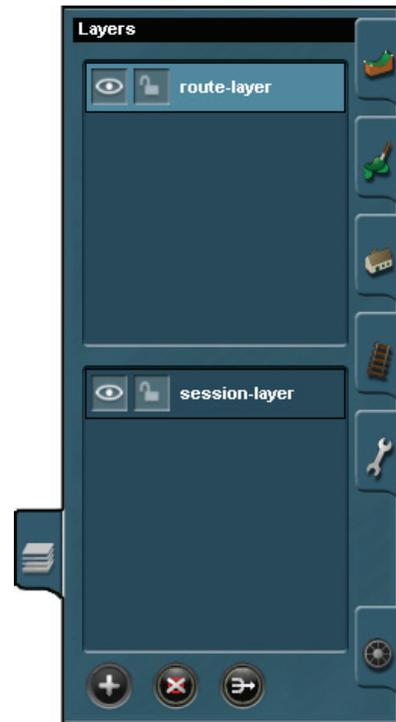
One of the advantages of using layers is the ability to set visible elements for a particular session, for example placing extra scenery or a side spur, which is specific to the session.
