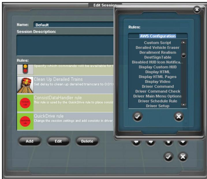
To allocate Drivers to various locos, click on Driver Set-up then Edit. You can also add Driver Commands for each Driver. R-Click on the small green arrow and choose a Command from the list. To add more Driver Commands to your list, edit the Driver Command Rule.
